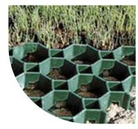
BODPAVE 40 porous grass pavers are an interlocking cellular paving grid system for grass and ground reinforcement applications where there is regular pedestrian or vehicle use. BODPAVE 40 permeable paving grids allow full rainwater penetration and are manufactured from UV stabilised 100% recycled HDPE, in black or green. BODPAVE 40 pavers are strong, chemically inert & non-toxic, enabling them to provide a durable, safe & sustainable eco-friendly surface for trafficked areas.
