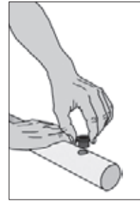
Remove shavings and place appropriate grommet firmly in hole with flange facing out
