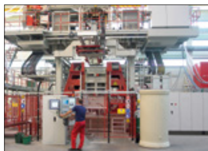
Blow moulding process
