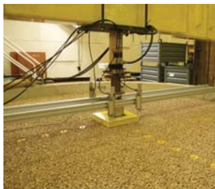
Bearing capacity tests at BRE confirm TriAx geogrids increase load distribution.
