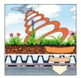
Planted areas are natural sound insulators and absorb more sound than hard surfaces. Green Roofs reduce reflective sound by up to 3 dB and improve sound insulation by up to 8 dB. This is very effective for buildings near airports, noisy nightclubs and factories.
