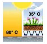
A Green Roof protects the waterproofing from climate extremes, UV exposure and mechanical damage. This greatly increases the life expectancy of the waterproofing and results in reduced maintenance and replacement costs.
