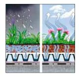
A Green Roof can reduce water run-off by 50-90%; any water flows from the roof with a delay. Outlets, pipes and drains can be reduced in capacity, thereby saving construction costs. Sewer costs can be reduced in some areas.
