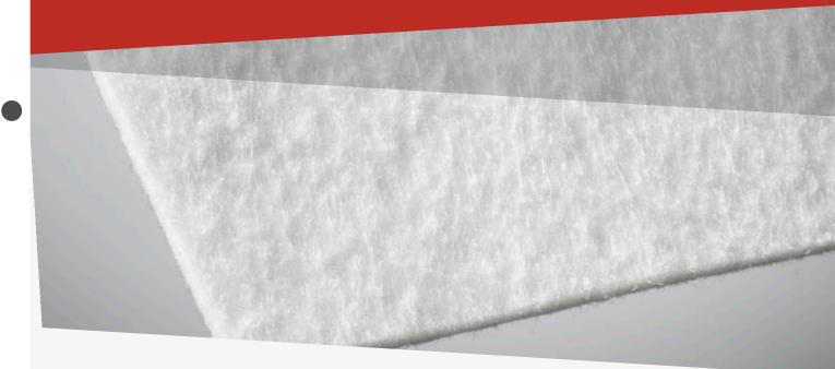
Bontec SNW (Superior Nonwoven Geotextile) is a needle-punched, lightly thermally bonded geotextile designed to offer outstanding performance at minimum weight. The SNW range offers superior puncture resistance when compared with most other needle-punched nonwoven products of comparable weight. Its principal functions are protection, separation and filtration.
