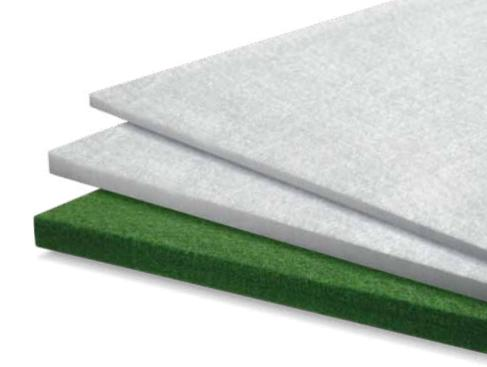
Nonwoven geotextile manufactured from UV stabilised, high tenacity, virgin polypropylene fibres that have been mechanically entangled to provide high strength, high extensibility, high loft and excellent abrasion characteristics.
